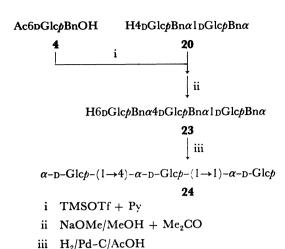
Fig. 1. Synthetic Scheme of α-Maltosyl α-p-Glucoside (24); Bn=-CH<sub>2</sub>Ph (cf. Ref. 19 for the code-expression of the protected carbohydrates).
